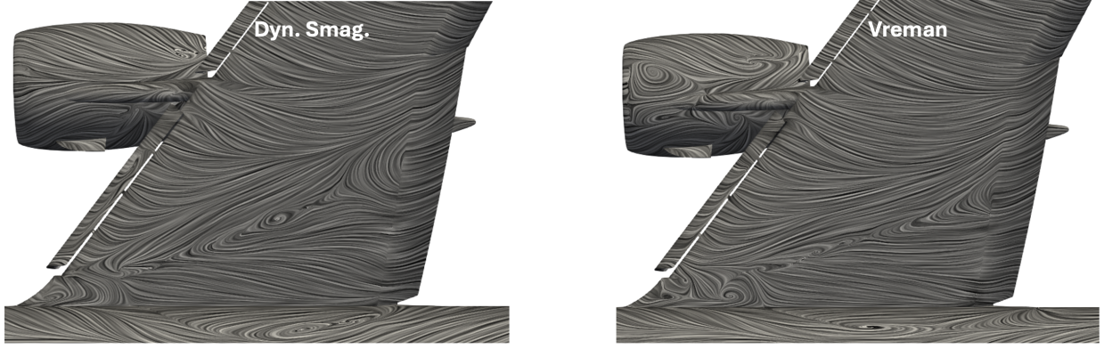
Fig. 31 Time-averaged surface streamlines showing sensitivity of subgrid-scale models at \alpha = 23.6^\circ for Case 2.4.
